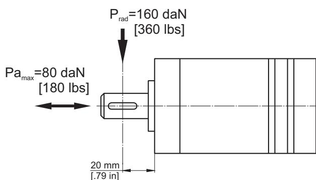
The permissible radial shaft load [ $P_{rad}$ ] is calculated from the distance [ $L$ ] between the point of load application and the mounting surface:
