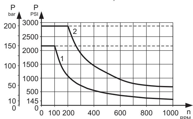
1: Curve for Standard Shaft Seal
