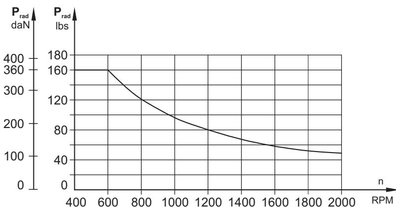
The drawing shows the permissible radial load when  $L=20$  mm [.79 in].
