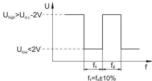
Load max.:  $I_{high} = I_{low} < 50mA$
