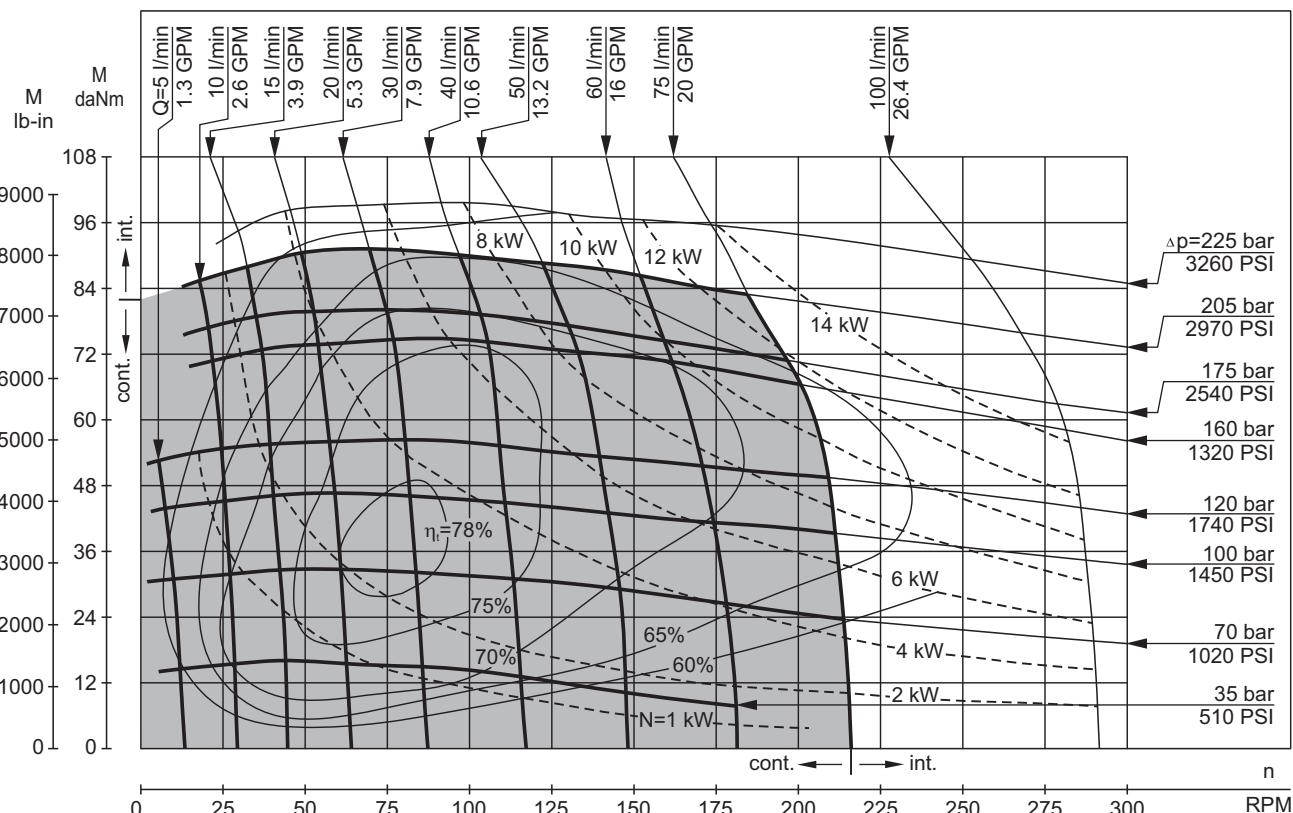
The function diagrams data is for average performance of randomly selected motors at back pressure  $5 \div 10$  bar [72.5 PSI  $\div$  145 PSI] and oil with viscosity of 32 mm<sup>2</sup>/s [150 SUS] at 50°C [122°F].
