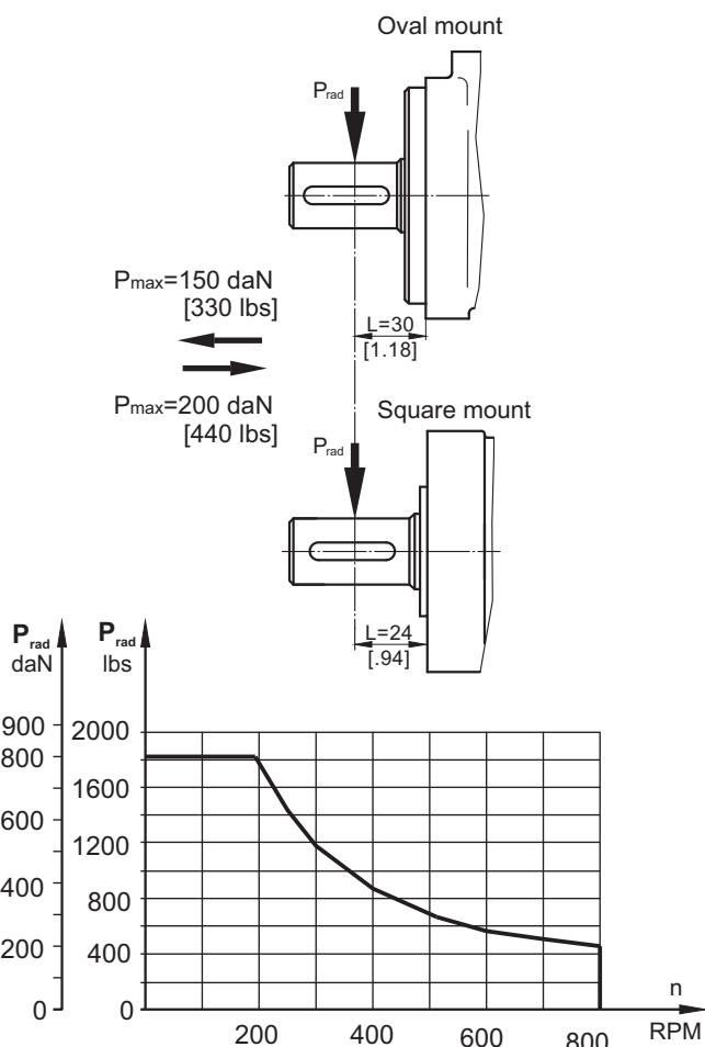
Radial Shaft Load  $P_{rad}$  for C, CO Shaft Extensions
