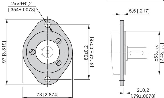
**F** Flange is mounted to the motor with 3 screws - M6x14. Tightening Torque: 5-6 Nm [44-53 lb-in].
