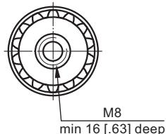
**CB** - ø35 straight, Parallel key A10x8x45 DIN 6885
