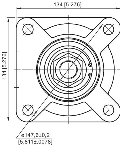
**V** Wheel mount, four holes, manifold 4xM6
