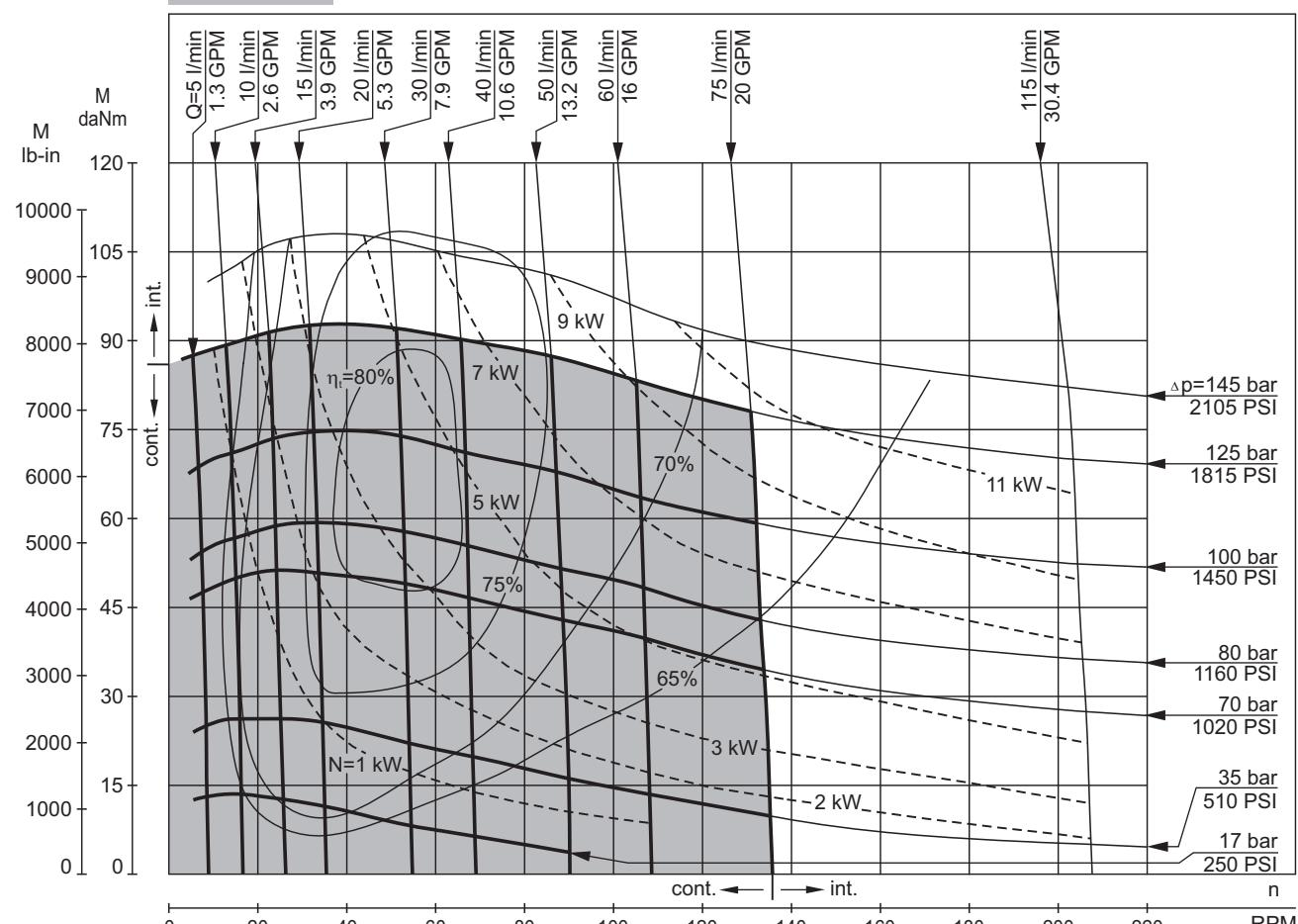
The function diagrams data is for average performance of randomly selected motors at back pressure  $5 \pm 10$  bar [72.5 PSI  $\pm$  145 PSI] and oil with viscosity of  $32 \text{ mm}^2/\text{s}$  [150 SUS] at  $50^\circ\text{C}$  [122°F].
