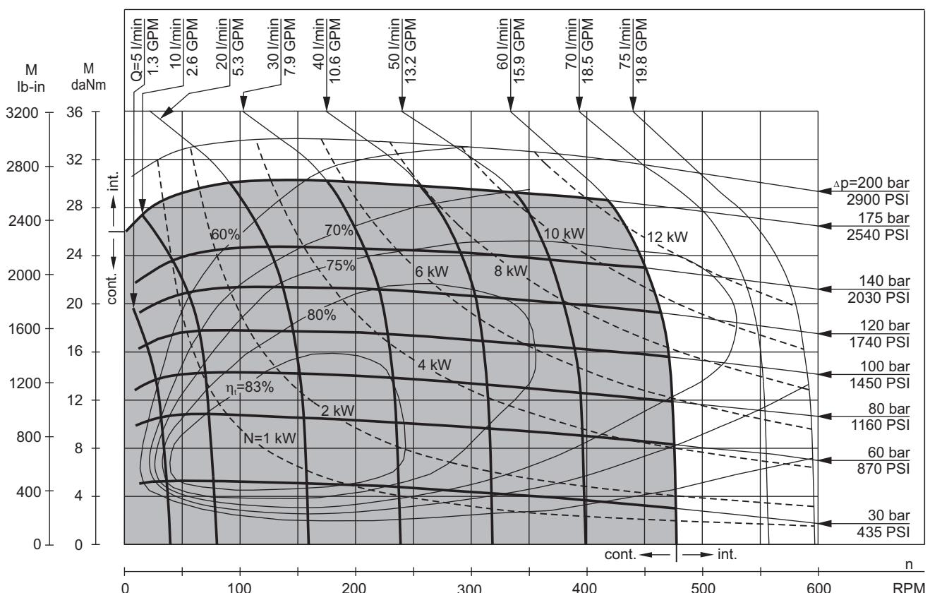
The function diagrams data is for average performance of randomly selected motors at back pressure 5÷10 bar [72.5 PSI÷145 PSI] and oil with viscosity of 32 mm<sup>2</sup>/s [150 SUS] at 50°C [122°F].
