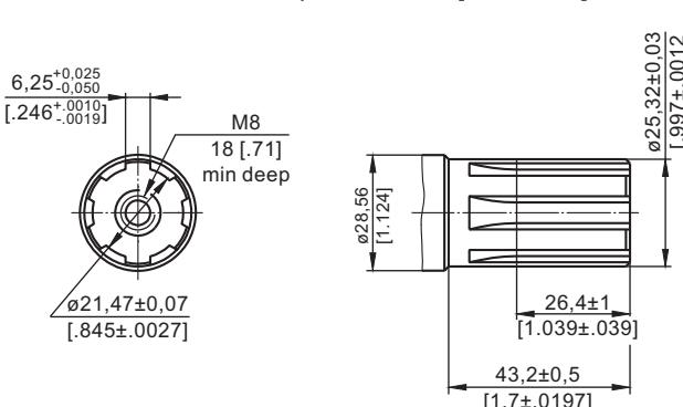
**K** - tapered 1:10, Parallel key B5x5x14 DIN 6885
