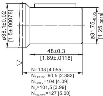
**M** - ø32 straight, Parallel key A10x8x32 DIN 6885
