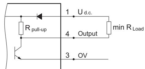
$$R_{Load} [\text{k}\Omega] = U_{d.c.} [\text{V}] / I_{max} [\text{mA}]$$
