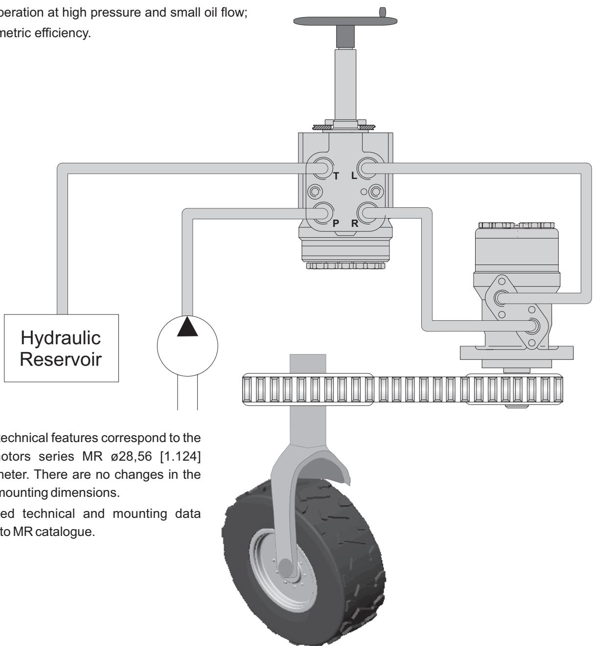
The main technical features correspond to the standard motors series MR ø28,56 [1.124] sealing diameter. There are no changes in the overall and mounting dimensions.
