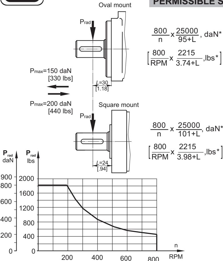
Radial Shaft Load  $P_{\text{rad}}$  for C, CO Shaft Extensions by  $L=30$  mm [1.18 in] (24 mm [.94 in])
