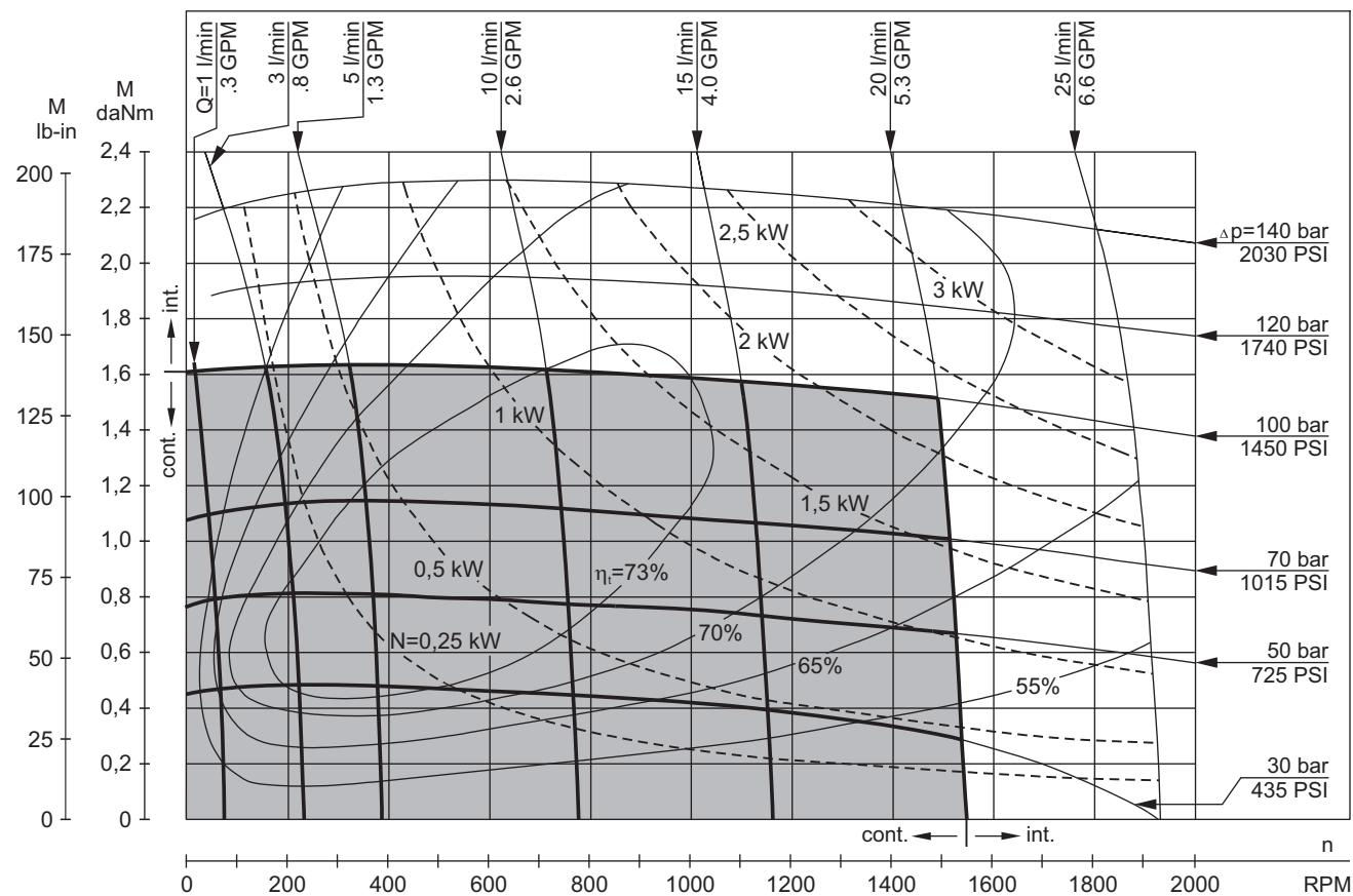
The function diagrams data is for average performance of randomly selected motors at back pressure 5÷10 bar [72.5 PSI÷145 PSI] and oil with viscosity of 32 mm<sup>2</sup>/s [150 SUS] at 50°C [122°F].
