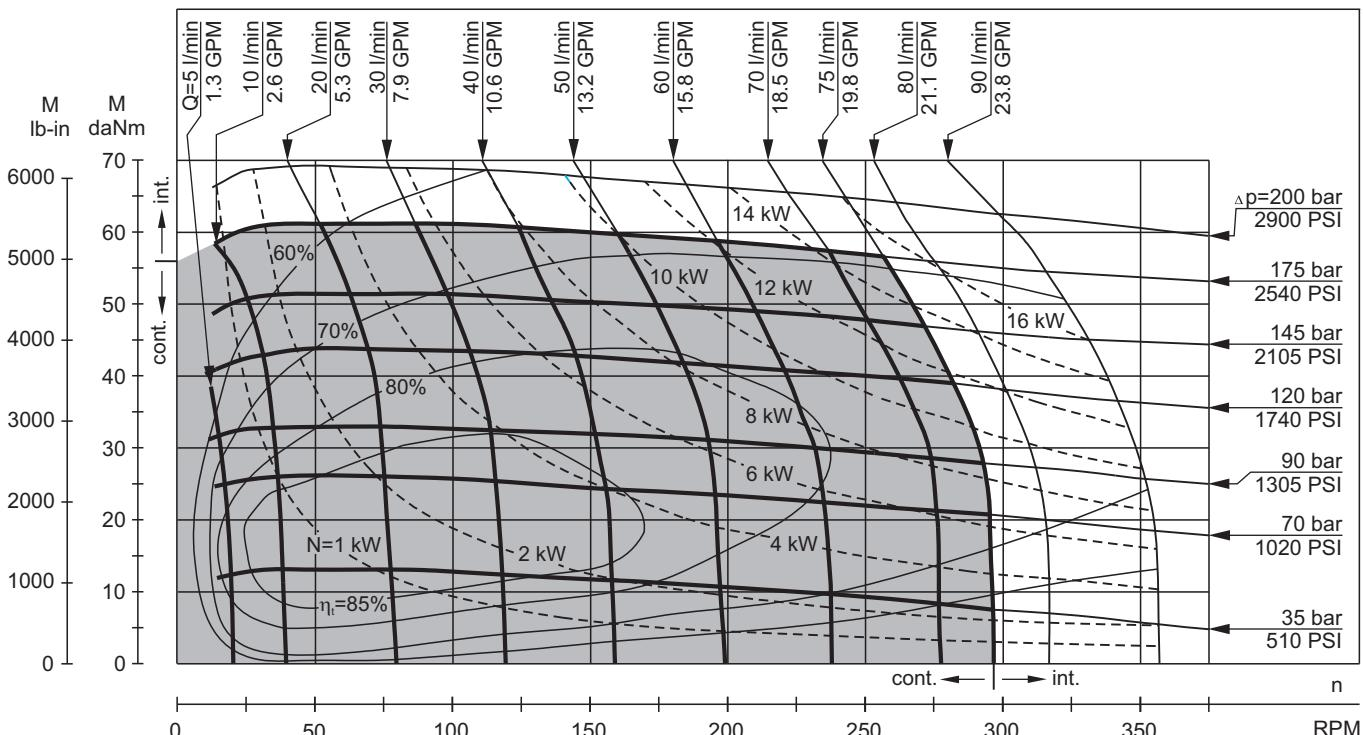
The function diagrams data is for average performance of randomly selected motors at back pressure 5÷10 bar [72.5 PSI÷145 PSI] and oil with viscosity of 32 mm<sup>2</sup>/s [150 SUS] at 50°C [122°F].
