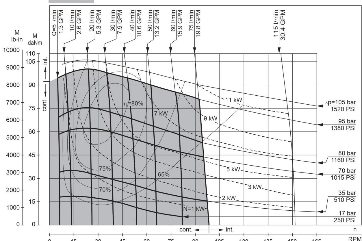
The function diagrams data is for average performance of randomly selected motors at back pressure  $5 \pm 10$  bar [72.5 PSI  $\pm$  145 PSI] and oil with viscosity of  $32 \text{ mm}^2/\text{s}$  [150 SUS] at  $50^\circ\text{C}$  [122°F].
