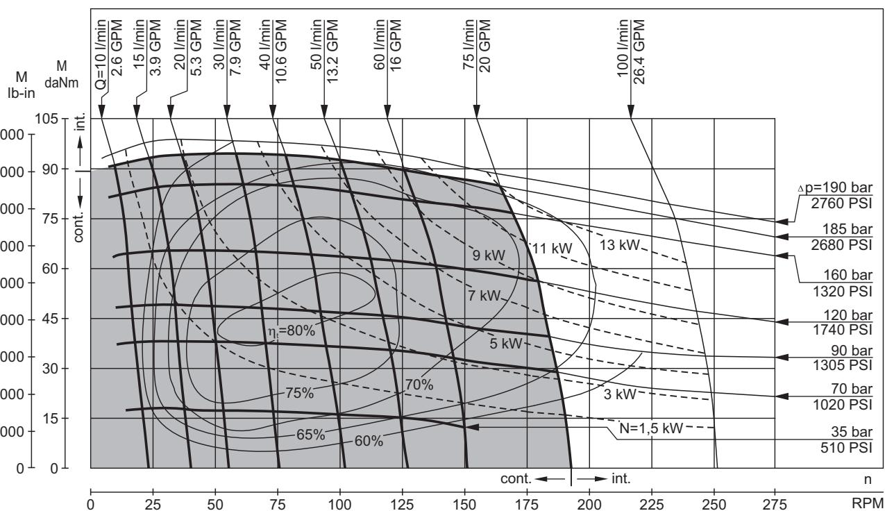
The function diagrams data is for average performance of randomly selected motors at back pressure 5÷10 bar [72.5 PSI÷145 PSI] and oil with viscosity of 32 mm<sup>2</sup>/s [150 SUS] at 50°C [122°F].
