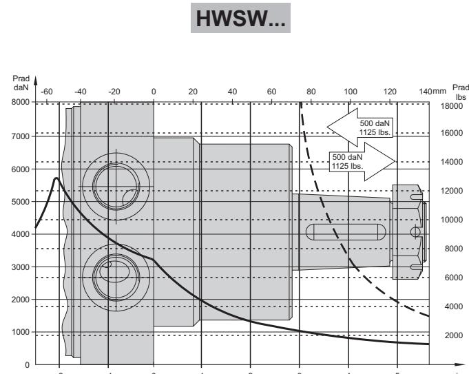
1 - Bearing curve: The curve applies to a B10 bearing life of 2000 hours at 100 RPM.
