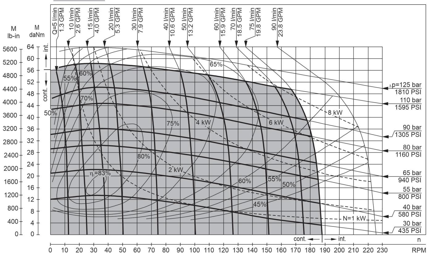
The function diagrams data is for average performance of randomly selected motors at back pressure 5÷10 bar [72.5 PSI÷145 PSI] and oil with viscosity of 32 mm<sup>2</sup>/s [150 SUS] at 50°C [122°F].
