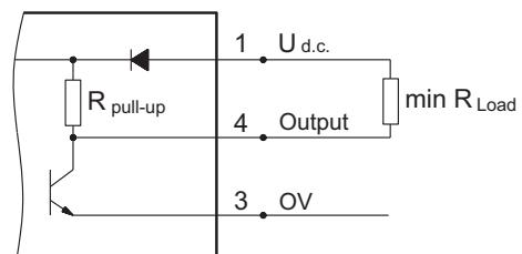
$$R_{\text{Load}} [\text{k}\Omega] = U_{\text{d.c.}} [\text{V}] / I_{\text{max}} [\text{mA}]$$
