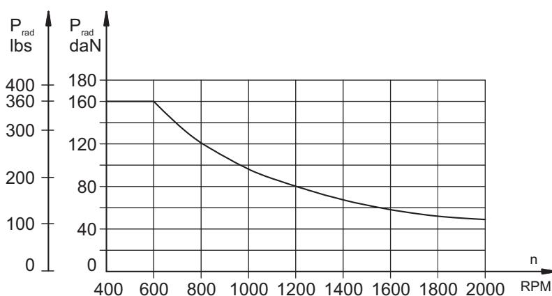
The drawing shows the permissible radial load when  $L= .79$  in [20 mm].
