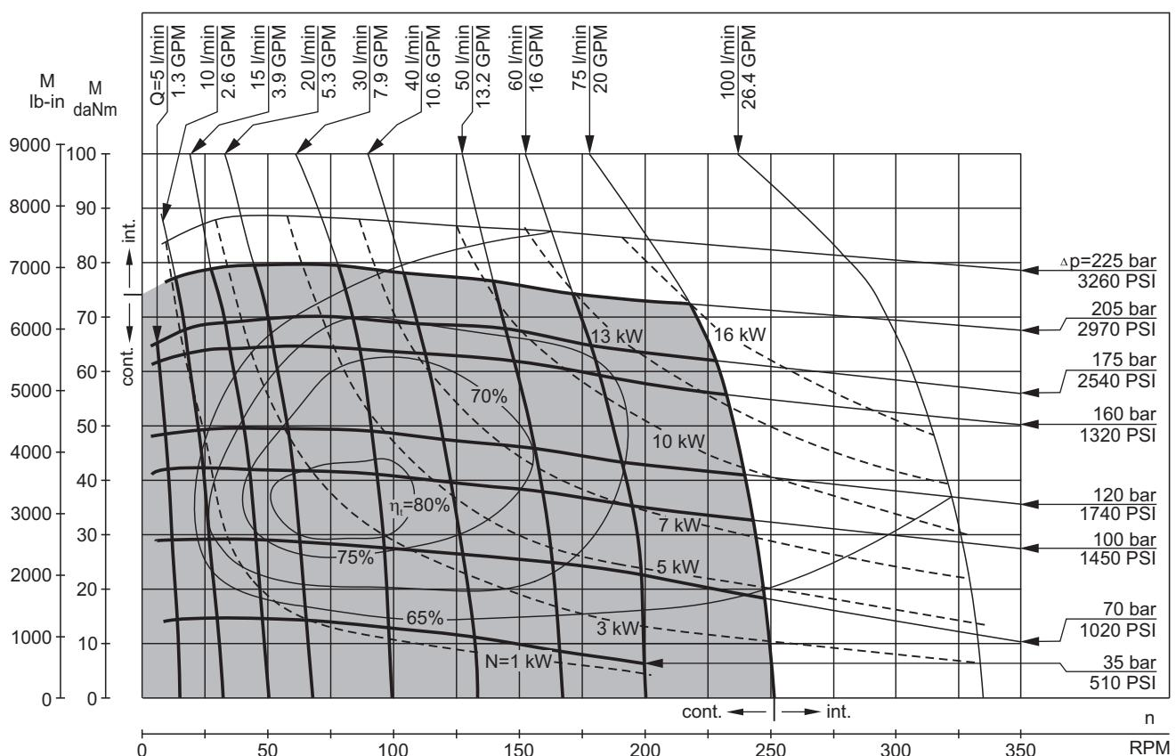
The function diagrams data is for average performance of randomly selected motors at back pressure 72.5 PSI $\pm$ 145 PSI [5 $\pm$ 10 bar] and oil with viscosity of 150 SUS [32 mm $^2$ /s] at 122°F [50°C].
