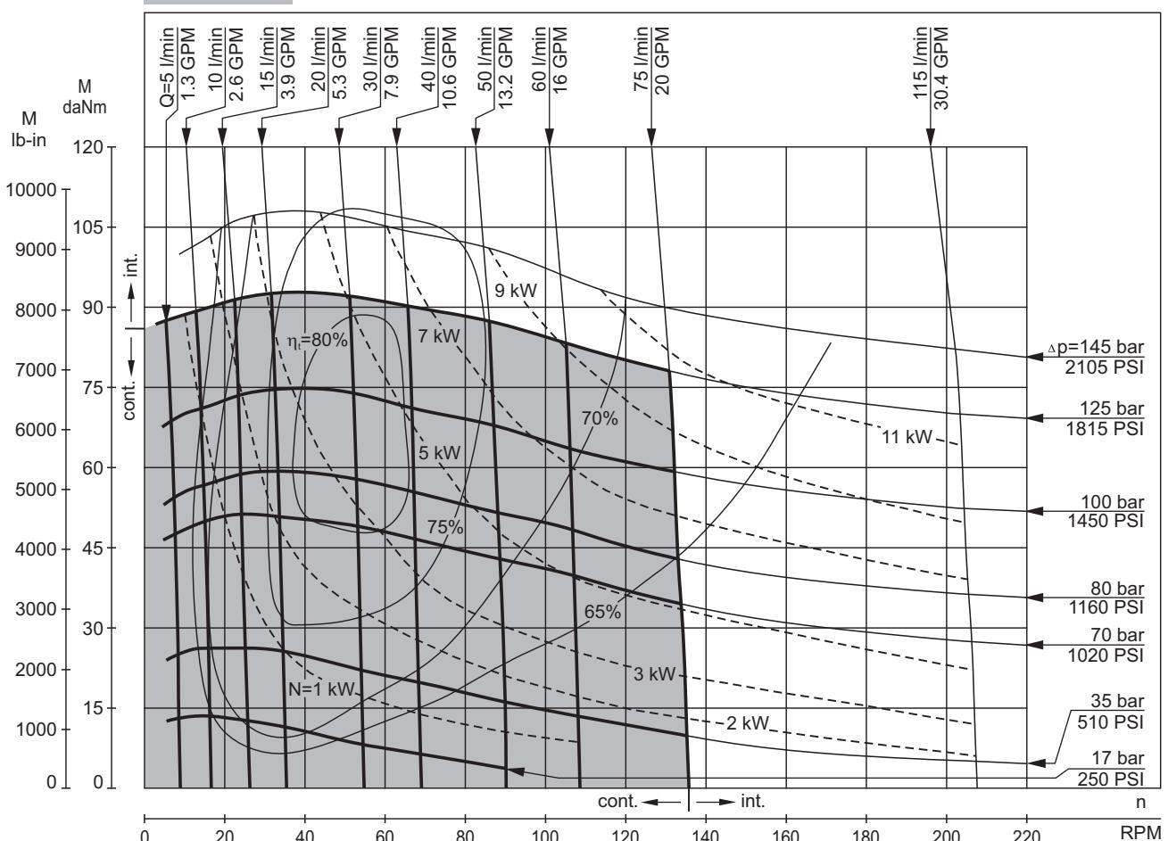
The function diagrams data is for average performance of randomly selected motors at back pressure 72.5 PSI/145 PSI [5±10 bar] and oil with viscosity of 150 SUS [32 mm<sup>2</sup>/s] at 122°F [50°C].
