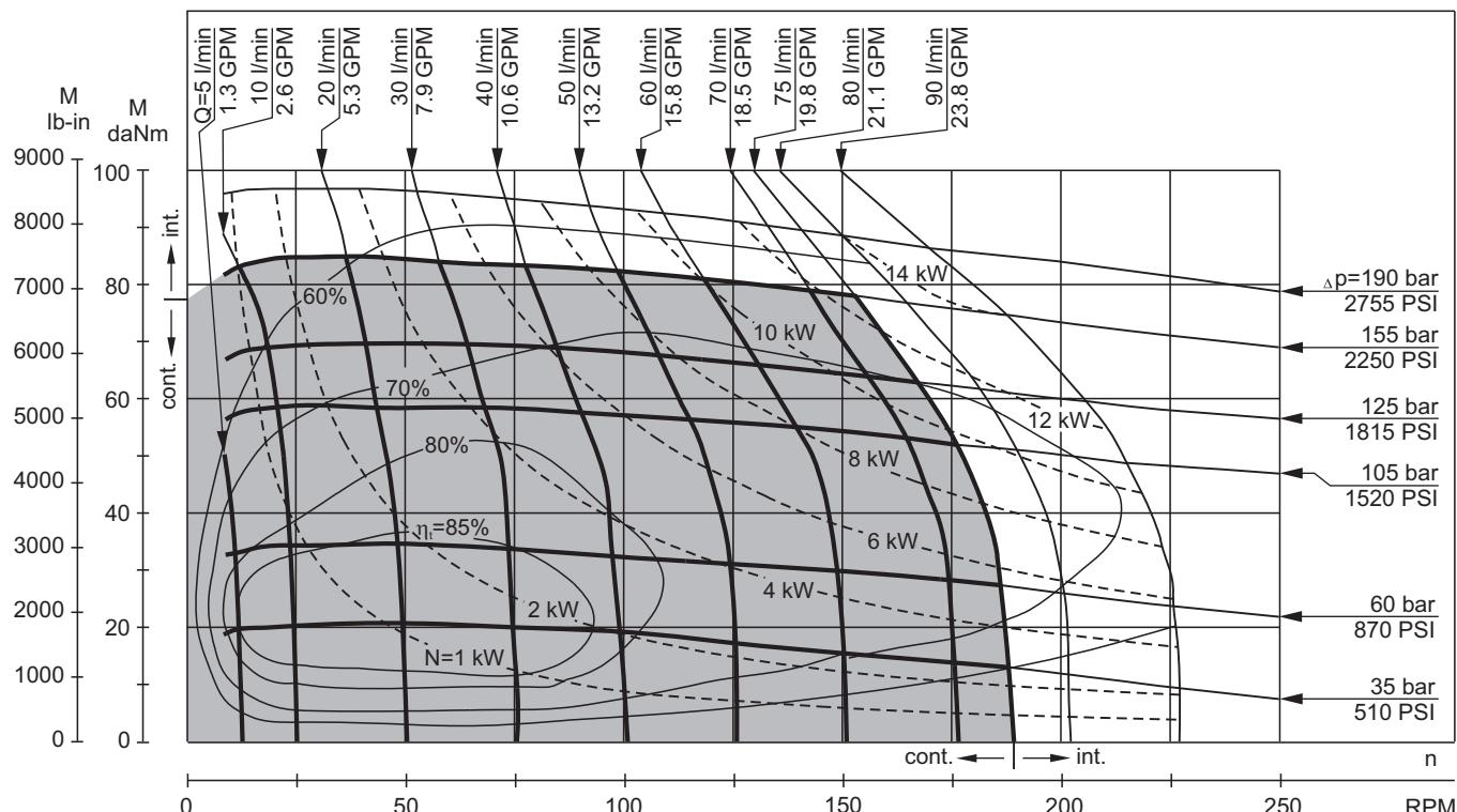
The function diagrams data is for average performance of randomly selected motors at back pressure 72.5 PSI +145 PSI [5+10 bar] and oil with viscosity of 150 SUS [32 mm<sup>2</sup>/s] at 122°F [50°C].
