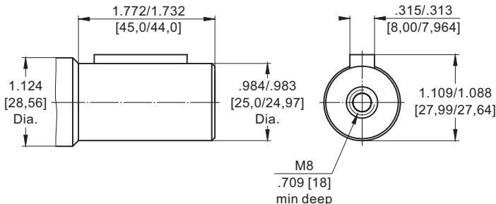
**CP** - ø25 straight, Parallel key A8x7x32 DIN 6885
