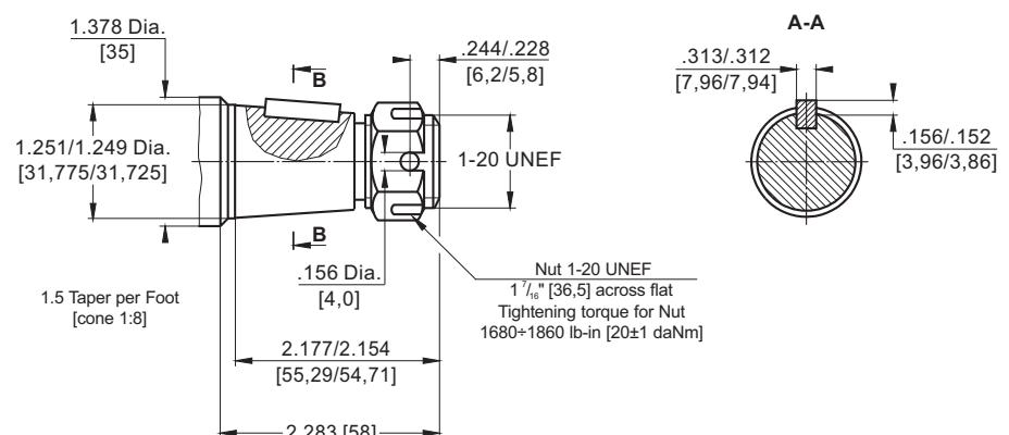
Requirement max. Torque must not be exceeded.
