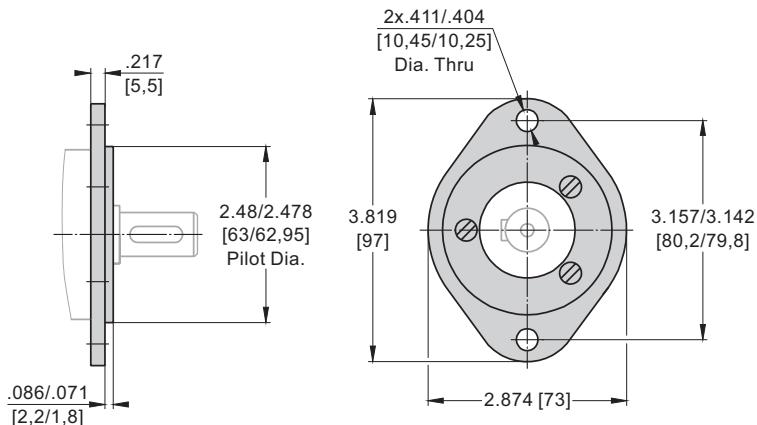
**F** Flange is mounted to the motor with 3 screws - 1/4-28 UNF.
