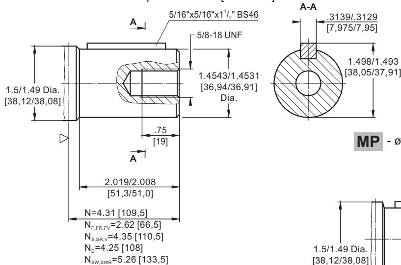
**MP** - ø32 straight, Parallel key A10x8x45 DIN 6885
