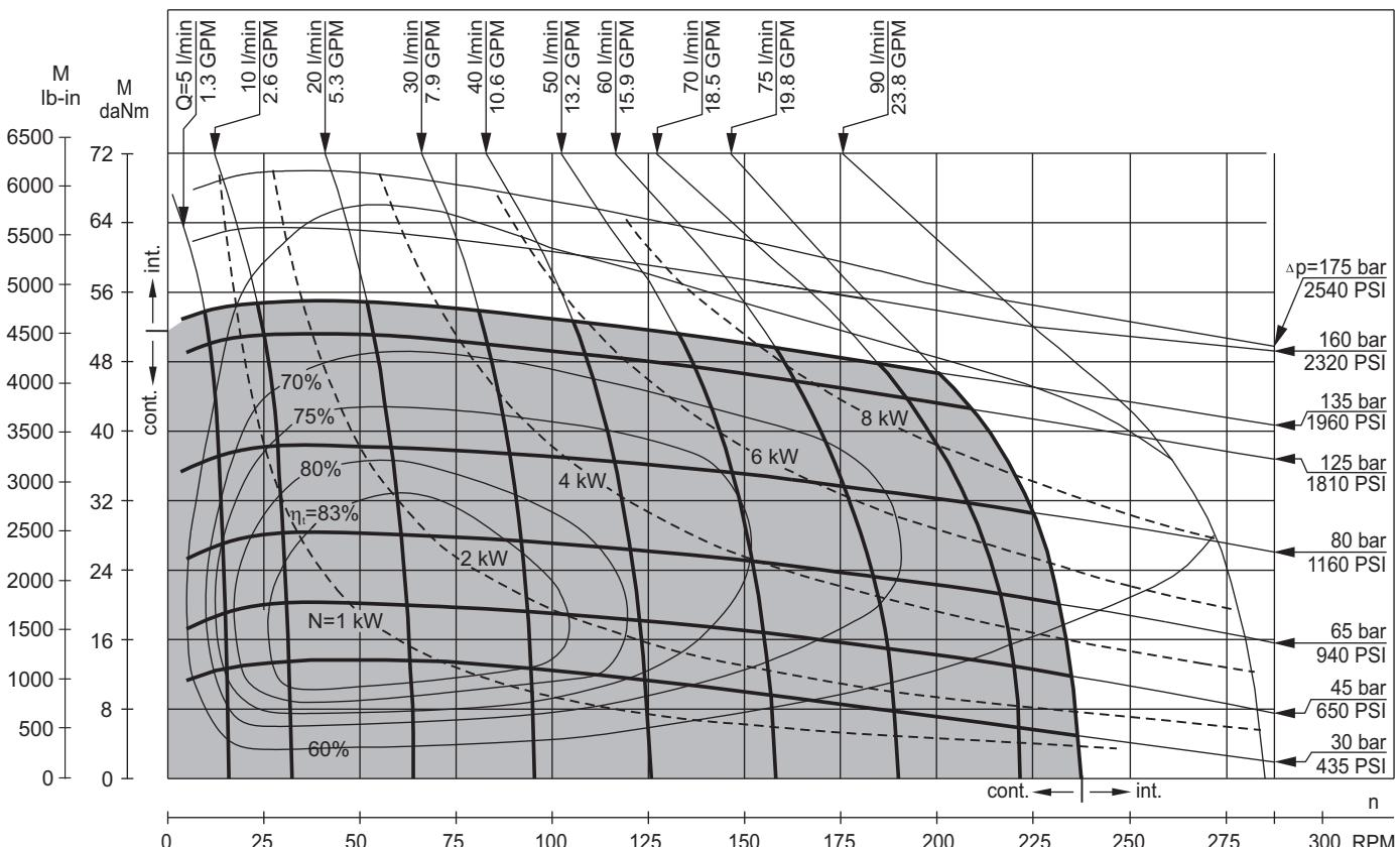
The function diagrams data is for average performance of randomly selected motors at back pressure 72.5 PSI÷145 PSI [5÷10 bar] and oil with viscosity of 150 SUS [32 mm<sup>2</sup>/s] at 122°F [50°C].
