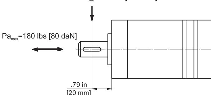
The permissible radial shaft load [ $P_{rad}$ ] is calculated from the distance [ $L$ ] between the point of load application and the mounting surface:
