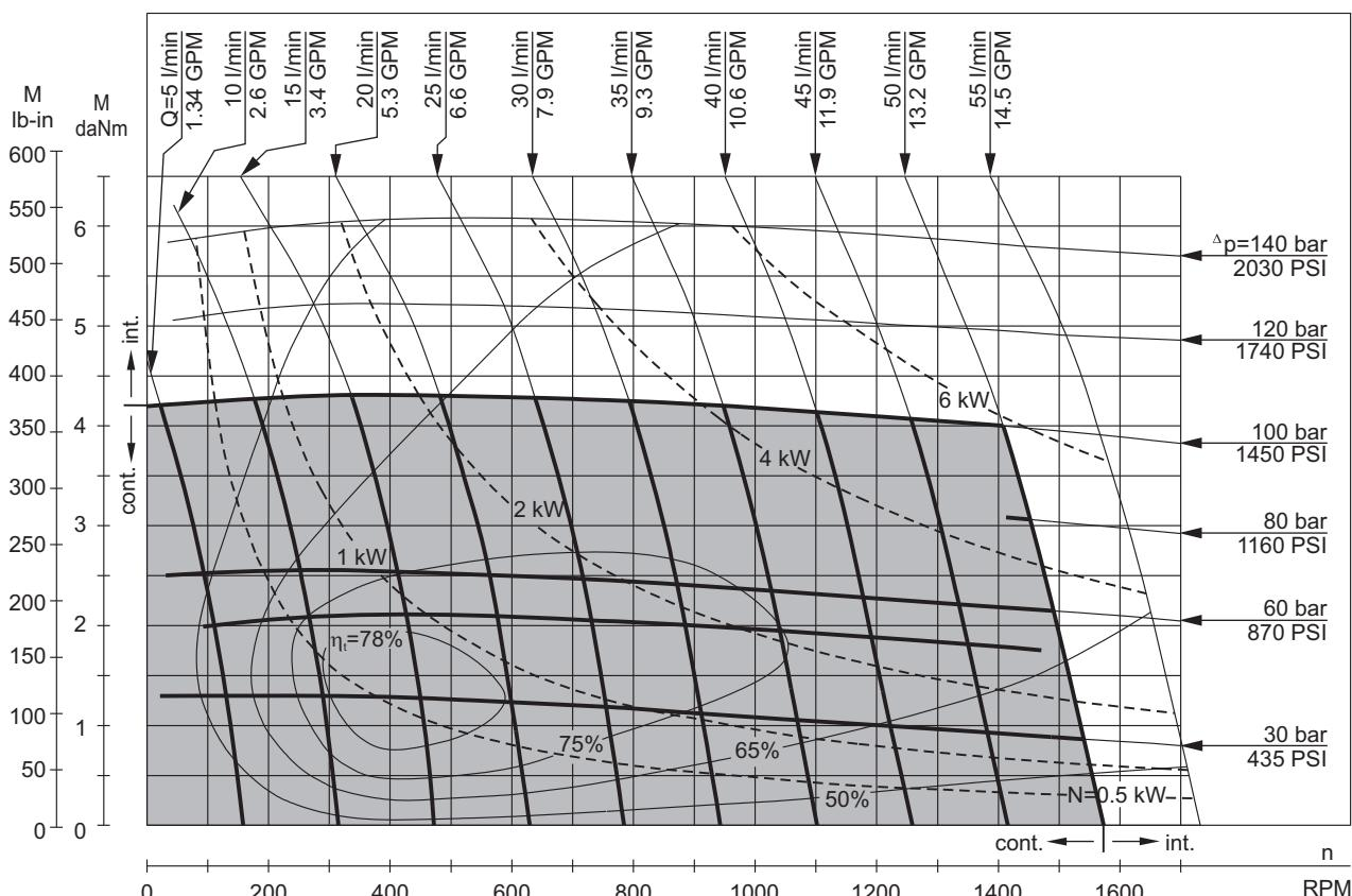
The function diagrams data is for average performance of randomly selected motors at back pressure 72.5 PSI +145 PSI [5+10 bar] and oil with viscosity of 150 SUS [32 mm<sup>2</sup>/s] at 122°F [50°C].
