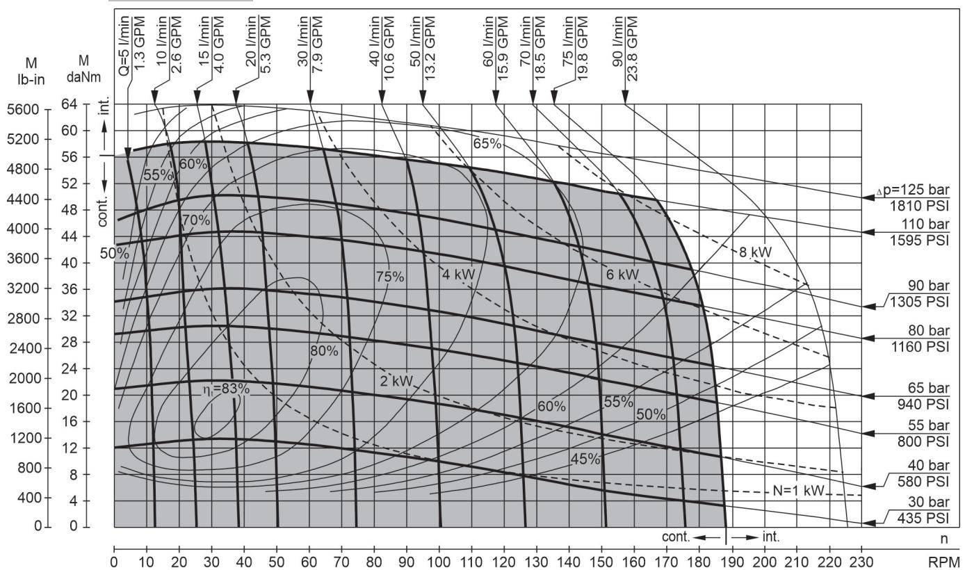
The function diagrams data is for average performance of randomly selected motors at back pressure 72.5 PSI÷145 PSI [5÷10 bar] and oil with viscosity of 150 SUS [32 mm<sup>2</sup>/s] at 122°F [50°C].
