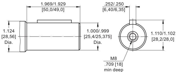
**CW** - ø25 straight, Parallel key A8x7x32 DIN 6885
